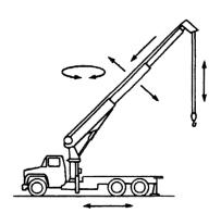
**Small Telescoping Boom Crane (Fixed Cab)**
