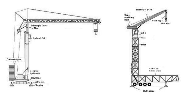
Types of Self-Erecting Tower Cranes Figure 44
