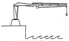
**Articulating Crane – Stationary Installation**
